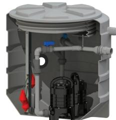
• Tank with pre-assembled hydraulics, 2 isolation valves and non-return valves, 3 floats installed in the tank, 1 or 2 Sanipump GR or VX, handling chain, waterproof terminal block, cable gland, Smart control box with alarm (with 2 pump versions)
