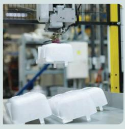
We have 42 injection moulding machines and 760 moulds within the factory. The production is fully automated, from taking the plastic pellets from silos right through to finished goods.
